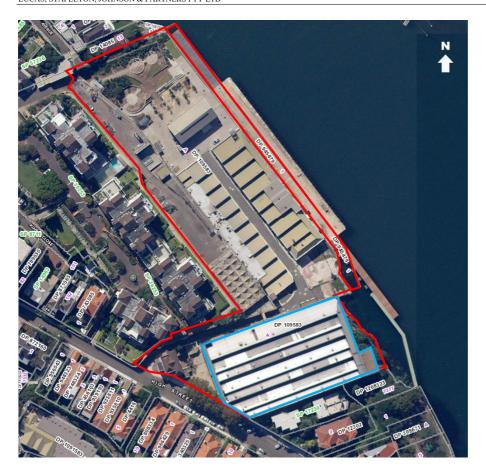
Figure 2: Aerial view of the locality showing the cadastral boundaries for the site and identifying the boundaries of the Harbour Trust land, including the land leased from RMS (in red). The Torpedo Factory is outlined in blue and is located in Lot A DP 109583. Source: NSW LPI, SixMaps
