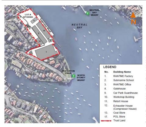
Figure 3: Extract from HMAS Platypus Management Plan identifying the boundaries of the site and the various buildings. The Torpedo Factory is identified as Building 1. Note buildings 3 and 9 have since been demolished. Source: Figure 1, *Management Plan* 2016
